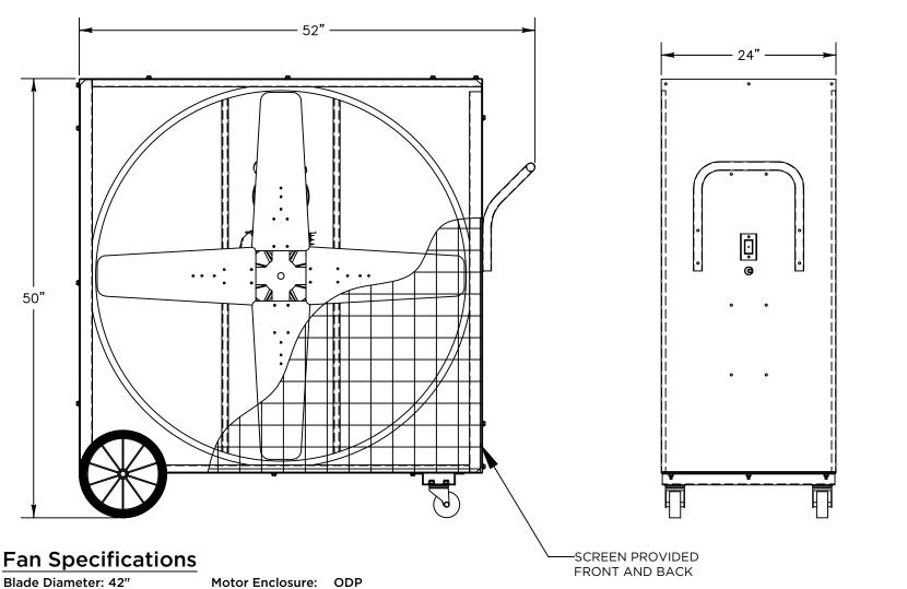
**Duty Cycle: Continuous Duty** Drive: Belt Horsepower: **OSHA Compliant** 1.5 **Guards:**
