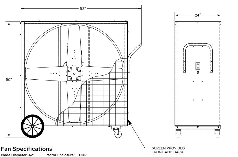
Drive: **Duty Cycle: Continuous Duty** Belt Horsepower: **OSHA Compliant Guards:** 1 10' with molded plug 230 Voltage: **Power Cord:**
