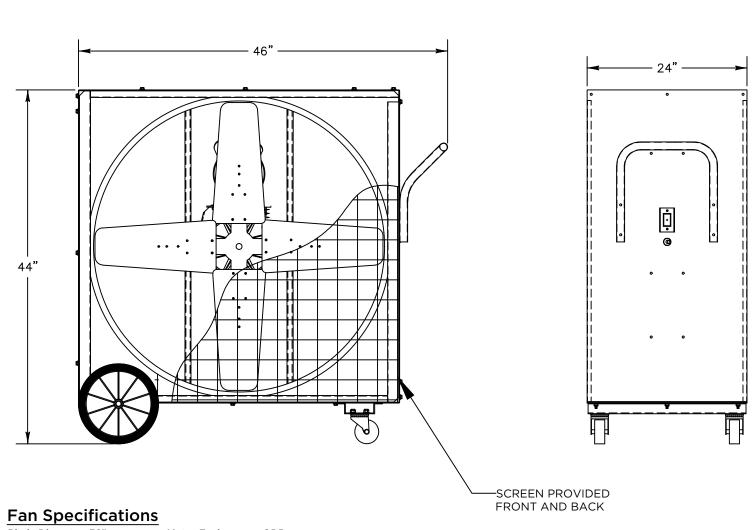
Blade Diameter: 36" Motor Enclosure: ODP
