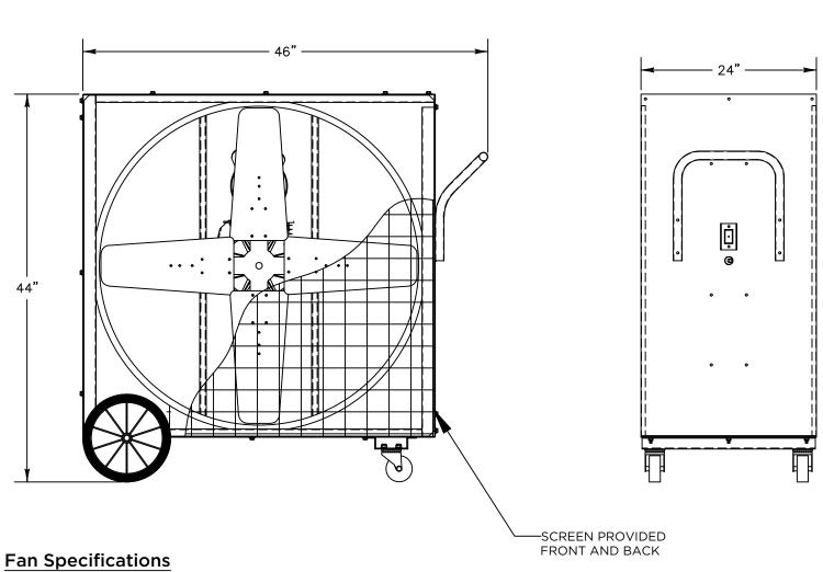
Blade Diameter: 36" Motor Enclosure: ODP
