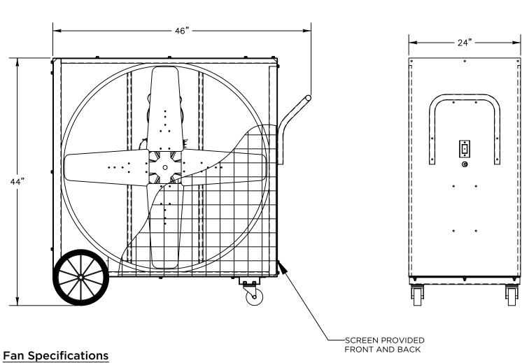
Blade Diameter: 36" Motor Enclosure: ODP
