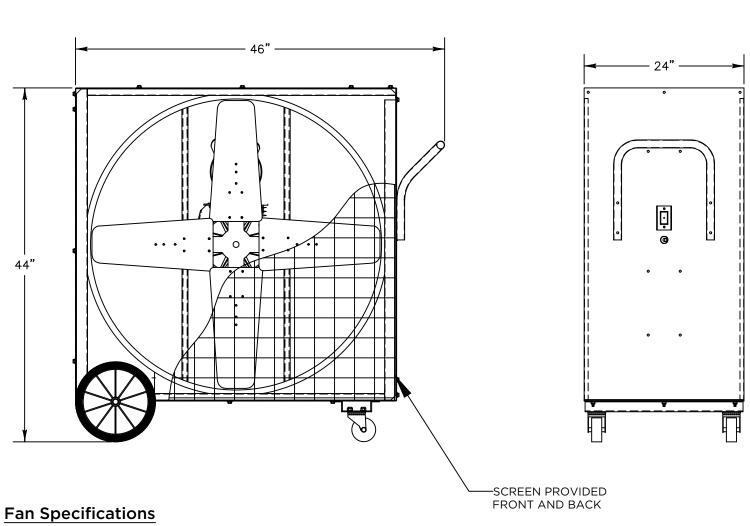
Blade Diameter: 36" Motor Enclosure: ODP
