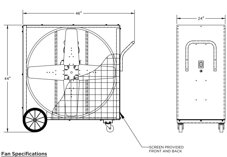
Blade Diameter: 36" Motor Enclosure: ODP
