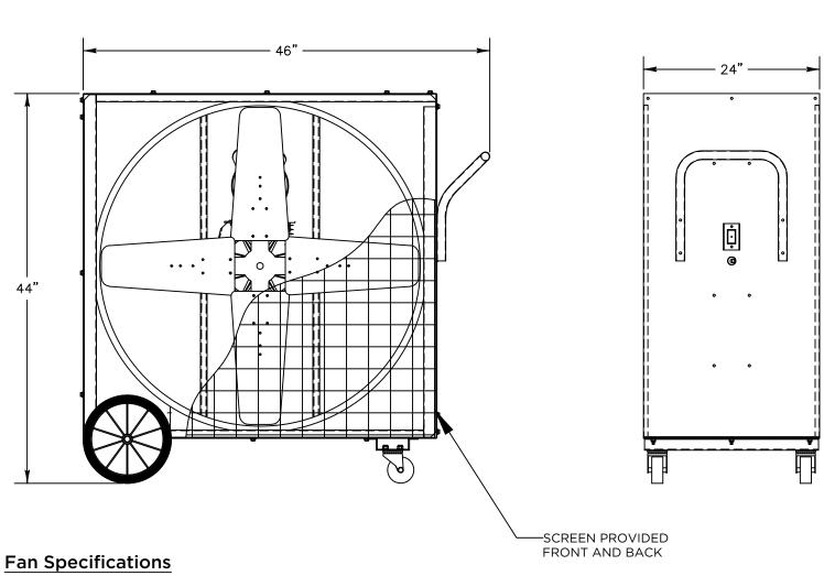
Blade Diameter: 36" Motor Enclosure: ODP
