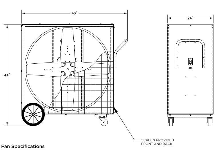
Blade Diameter: 36" Motor Enclosure: ODP
